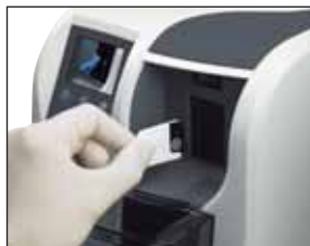
Automatic opening of the entry slot
